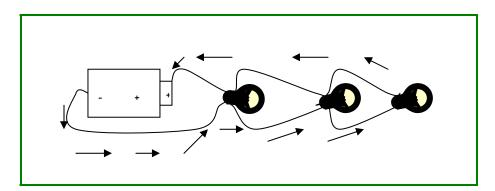
Batteries in a series: are two or more batteries connected to make a circuit. The negative electrode of one battery is connected to the positive electrode of the next battery. Batteries in a series will increase the voltage (there will be more electricity flowing).
