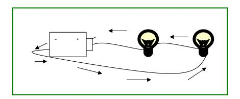
• Parallel Circuits: are constructed with two wires running side by side. When one light goes out in a parallel circuit, the other lights remain illuminated.
