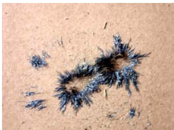
Iron filings under magnetic field
